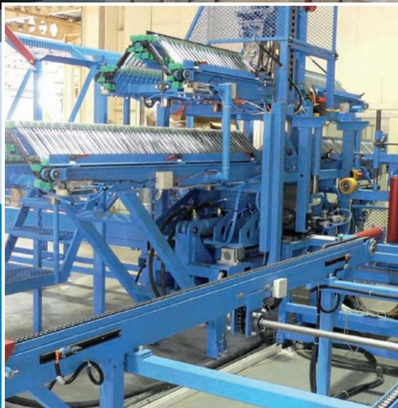
The ReVolution has a unique and patented vertical pressing station with CNC controlled positioning of the Posi-Strut™ webs ensuring precise and accurate placement every time and eliminating lengthy setting up procedures. Capable of over 1500m in a single shift.
